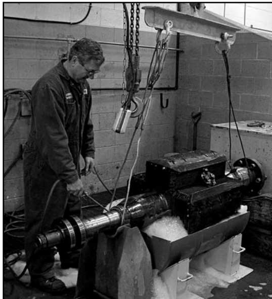
Brother Frank Bianci looks over the "bubble cleaning" of an armature.
